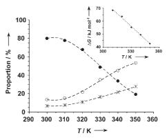
Figure 10. Speciation in solution diagram as a function of temperature. ( •)  $[Mo_{16}(IsoP)_2]^{4-}$ ; ( $\bigcirc$ )  $[Mo_{12}IsoP]^{2-}$ ; (\*) free ligand  $IsoP^{2-}$ . Dotted lines are only guides for eyes. Insert: Variation of  $\Delta_r G^+$  as a function of temperature.
